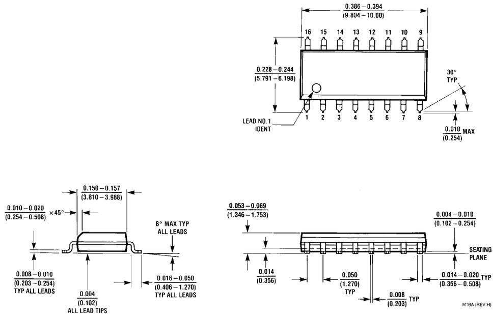
**16-Lead Small Outline Integrated Circuit (SOIC), JEDEC MS-012, 0150<sup>th</sup> Narrow Body
