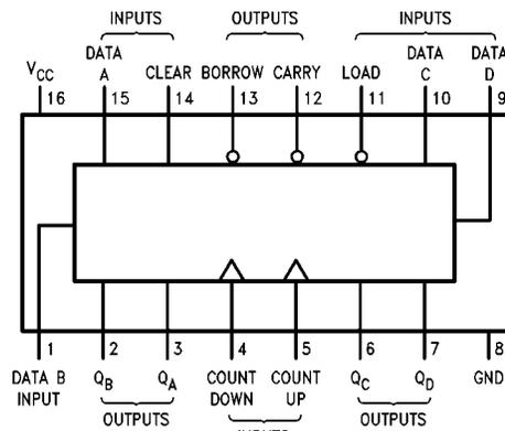
DM74LS193 Synchronous 4-Bit Binary Counter with Dual Clock
