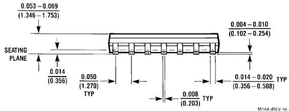
**14-Lead Small Outline Integrated Circuit (SOIC), JEDEC MS-120, 0.150" Narrow
