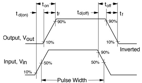
Figure 12. Switching Waveforms.
