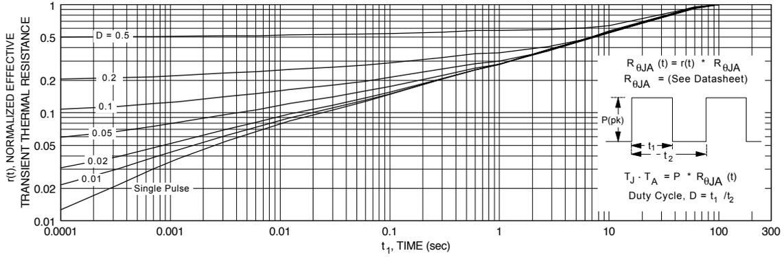
Figure 15. TO-92, BS170 Transient Thermal Response Curve.
