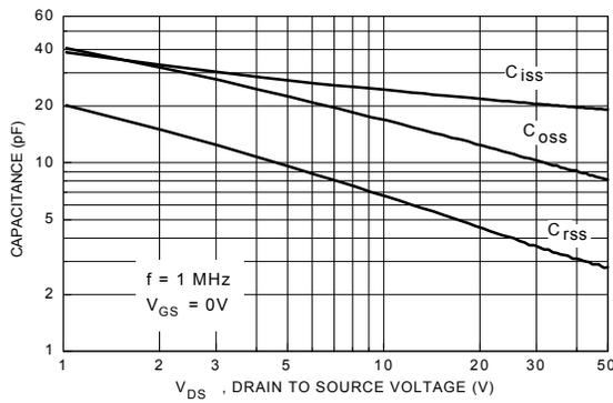
Figure 9. Capacitance Characteristics.
