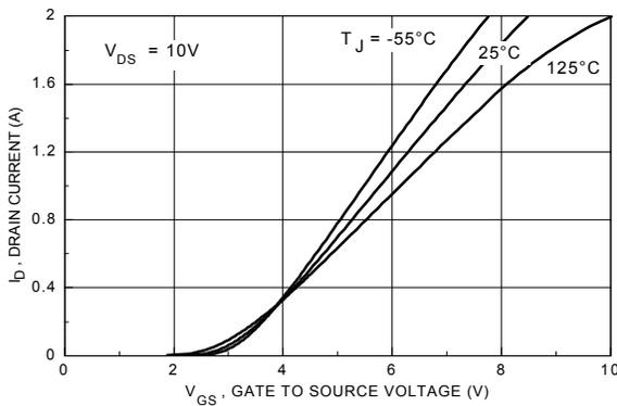
Figure 5. Transfer Characteristics.
