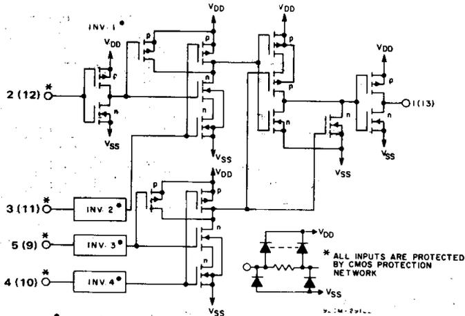
Fig. 7 - Schematic diagram for CD4072B (1 of 2 identical gates).
