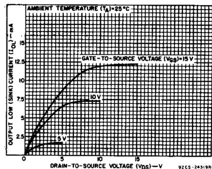
Fig. 6 - Minimum output low (sink) current characteristics.
