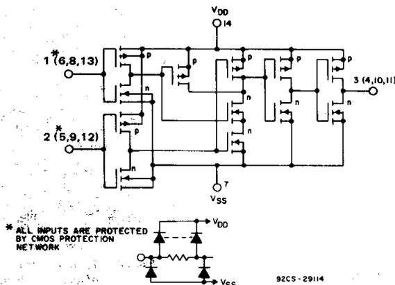
Fig. 3 - Schematic diagram for CD4071B (1 of 4 identical gates).
