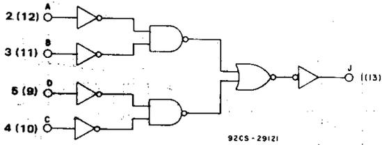
Fig. 9 - Logic diagram for CD4072B (1 of 2 identical gates).
