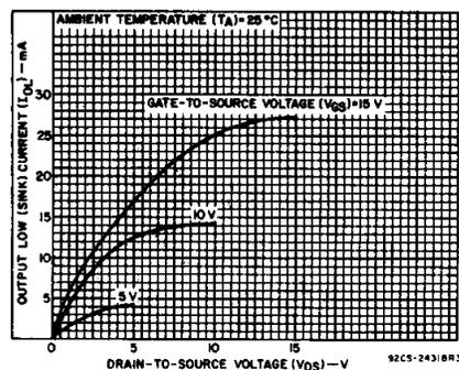
Fig. 4 - Typical output low (sink) current characteristics.
