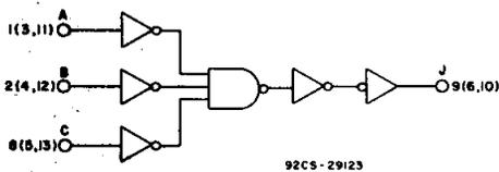
Fig. 13 - Logic diagram for CD4075B (1 of 3 identical gates).
