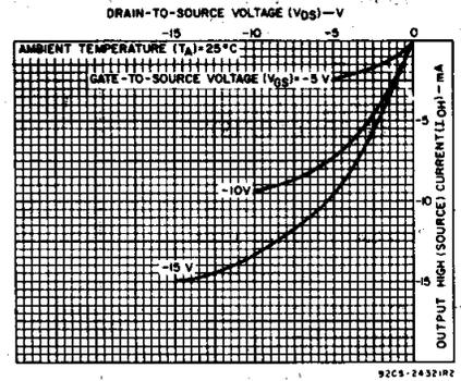
Fig. 10 - Minimum output high (source) current characteristics.
