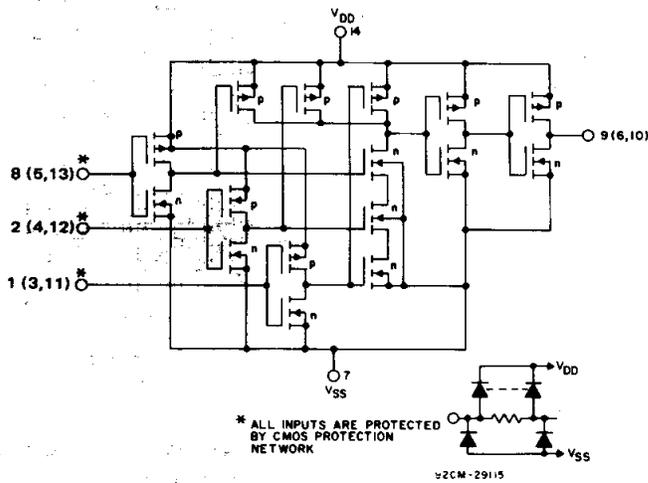
Fig. 11 - Schematic diagram for CD4075B (1 of 3 identical gates).
