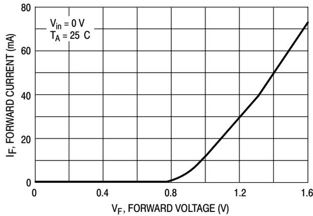
**Figure 8. Clamp Diode Forward Current versus Voltage**
