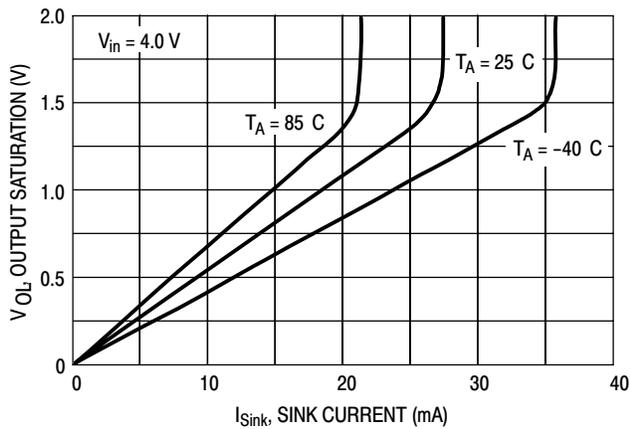
Figure 6. Reset Output Saturation versus Sink Current
