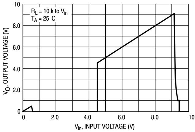
Figure 2. Reset Output Voltage versus Input Voltage
