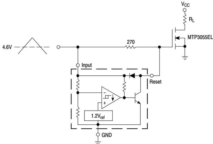
Overheating of the logic level power MOSFET due to insufficient gate voltage can be prevented with the above circuit. When the input signal is below the 4.6 V threshold of the MC34064, its output grounds the gate of the L<sup>2</sup> MOSFET.
