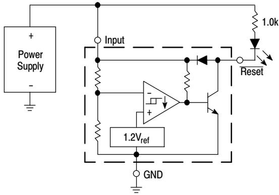
Figure 11. Voltage Monitor
