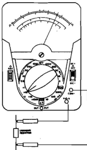
Fig. 4 Measuring DC Resistance
