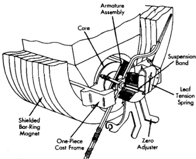
2. Greater ruggedness and durability as no moving parts are in contact and the elimination of the hairspring prevents snagging and tangling. The tension spring acts as a built-in shock absorber.
